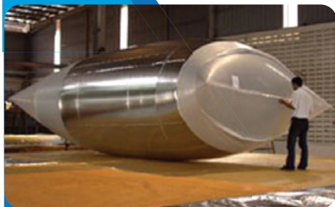
Each heat seal is tested to 120% of load capacity
