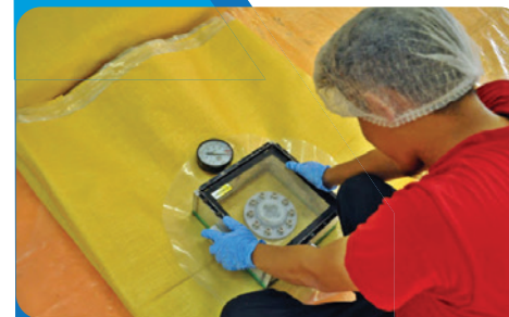
Each load & discharge fitting is vacuum tested
