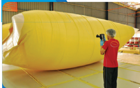
Each flexitank is ultrasonic tested to be leak proof
